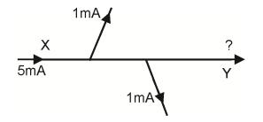
Here is part of an electric circuit. Electric current is measured in units called milliamps, (mA).
