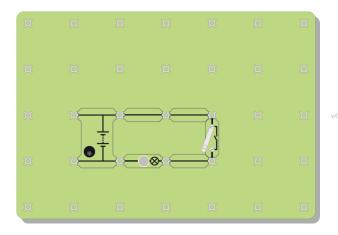
Change the circuit so that there are two bulbs in it, and the switch controls both bulbs.
