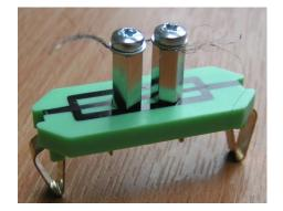
Tease out one or two strands of wire wool from the pack. Carefully clamp them across the gap of the sampler, as shown in the photograph.
