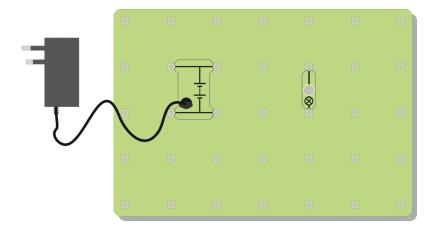
You have just used two circuit symbols, one standing for a battery, or group of batteries, and the other for a lamp, or sometimes any kind of indicator.
