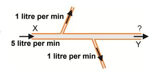
Here is a pipe, carrying water. It does not leak! Five litres of water enter the pipe at X every minute. Some water flows down the side pipes, as shown. How many litres per minute leave the pipe at Y?
